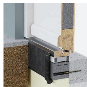
passive system (threshold)
