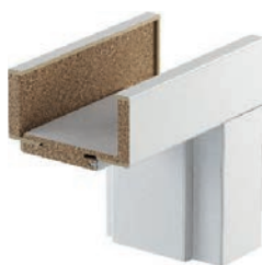
door frame profile – 80 mm architrave for door height 2.0 – 100 mm mm architrave for door height 2.2
