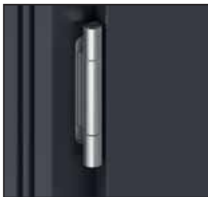
Premium Simonswerk hinges series 4000 • 3D regulation • carrying capacity 160 kg • anti-burglary reinforced • 30 years functioning guarantee (200 thousand cycles)
