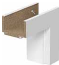
door frame profile – architrave 80 mm for doors height 2.0 – architrave 100 mm for doors height 2.2
