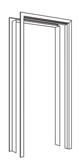
2 - piece (covering) for assembly on masonry walls, concrete and plasterboard walls
