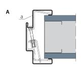
A. Method of anchoring to light door leaves a) assembly on plasterboard wall with clamping anchors [a] bolted with screws
