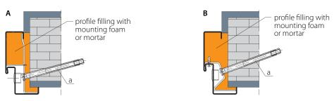
a) assembly of ROMA Standard folded door frames with metal dowels [a] and mouting foam or mortar b) assemby of PORTA SAFE folded door frames with metal dowels [a] and mounting foam or mortar
