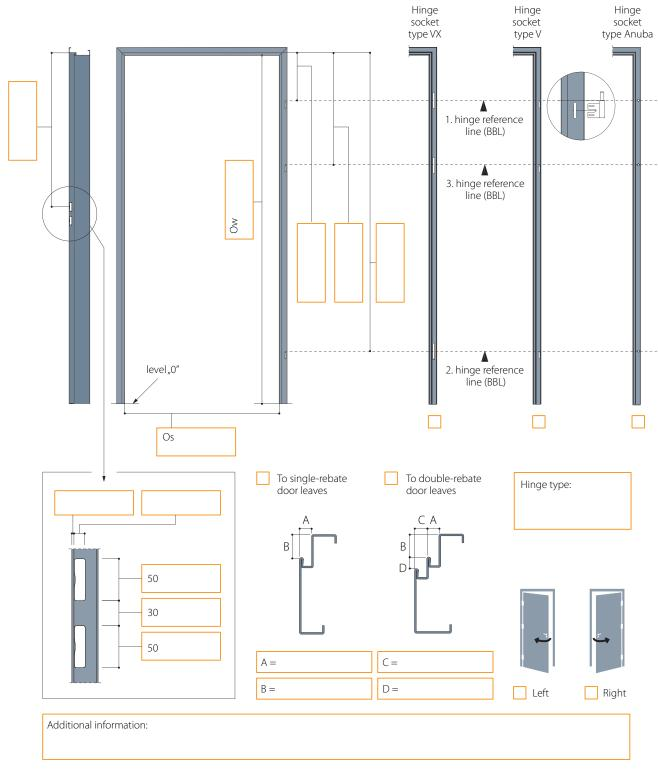
Ow - height of clear opening in door frame Os - width of clear opening in door frame
