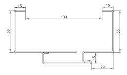
Adjustable PS door frame with sharp edges
