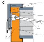
profile filling with plasterboard strips 9,5 mm thick, made during the assembly on a site
